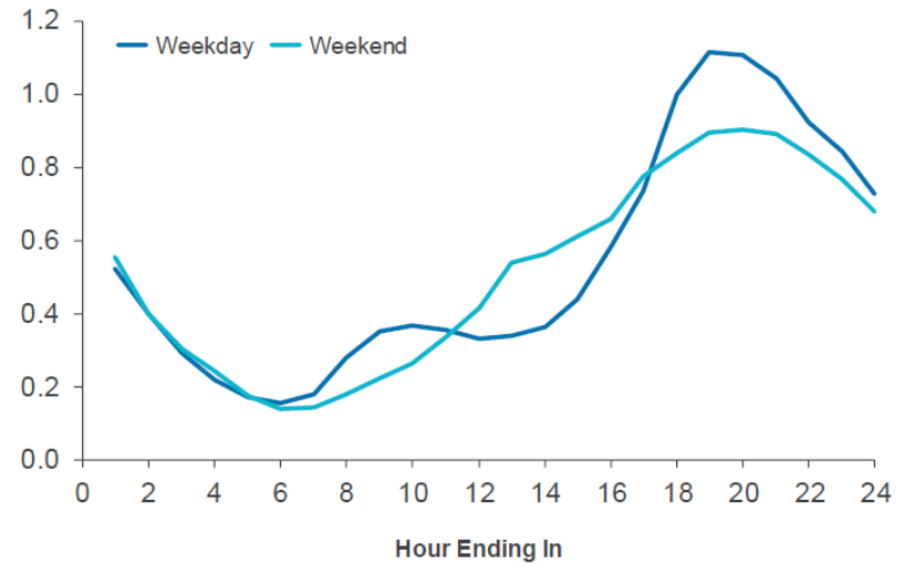
EV load shapes assumed in BELCo's Integrated Resource Plan, based on U.S. Department of Energy Alternative Fuel Data Centre model for Kahului. © Charles Rivers Associates
